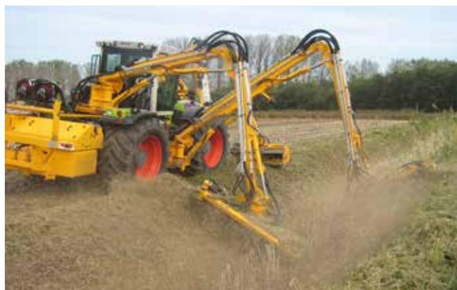
Four mowing arms on one tractor. We don't build this kind of machine every day. The machine was developed to mow the slope on its own side, the slope on the other side, shoulder on its own side and the vegetation above the water level in one run. Quattro à la Herder.
