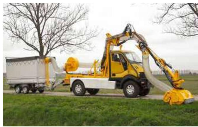
Herder developed this machine for working on road shoulders with minimal traffic measures.
