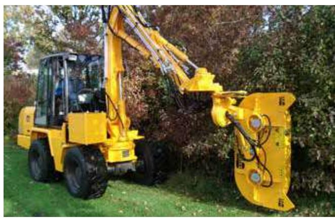
Herder develops machines based on a wide range of vehicles. This example shows a loader as the basis. The removal of the original loading boom made the vehicle suitable for vegetation maintenance, for instance.
