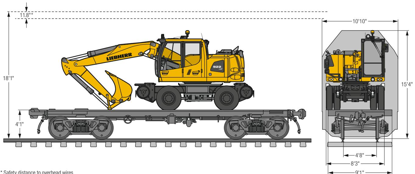
\* Safety distance to overhead wires
