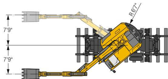
\* Safety distance to overhead wires
