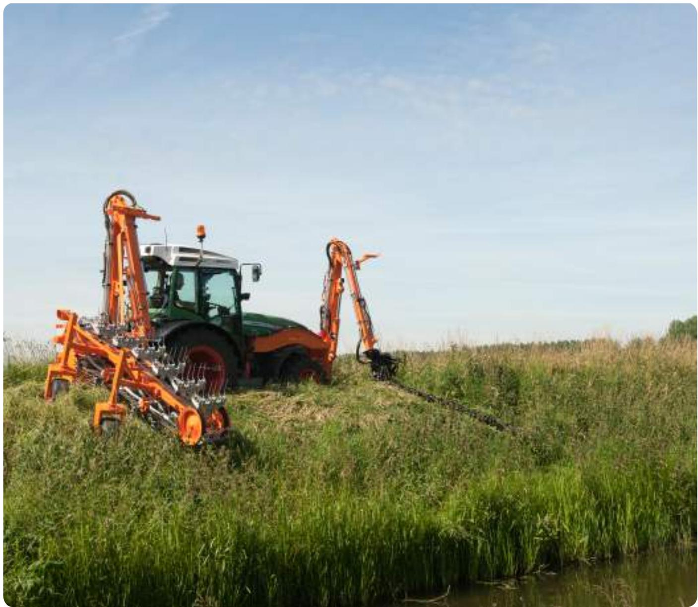
Complete the entire ditch maintenance from the tow path in one run in the most environmentally-friendly way possible? It can be done, simply and fast, with the Conver C36 mower-rake combination. The front end of a tractor is equipped with a mowing unit and the rear with a raking unit.
